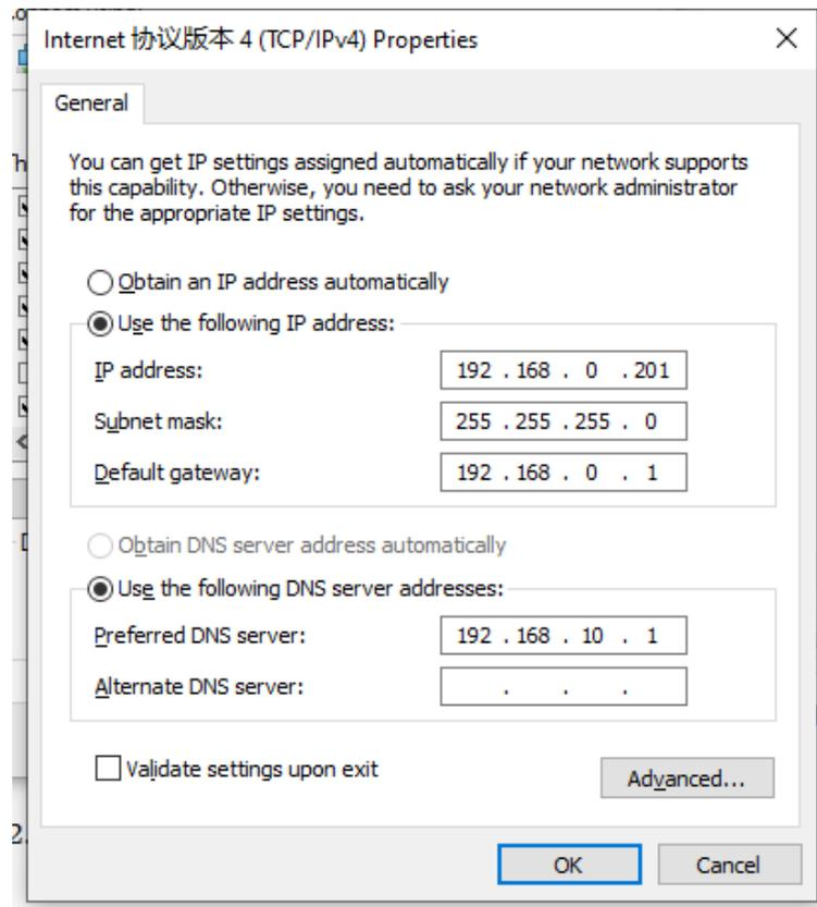
Figure 1 computer IP address configuration
