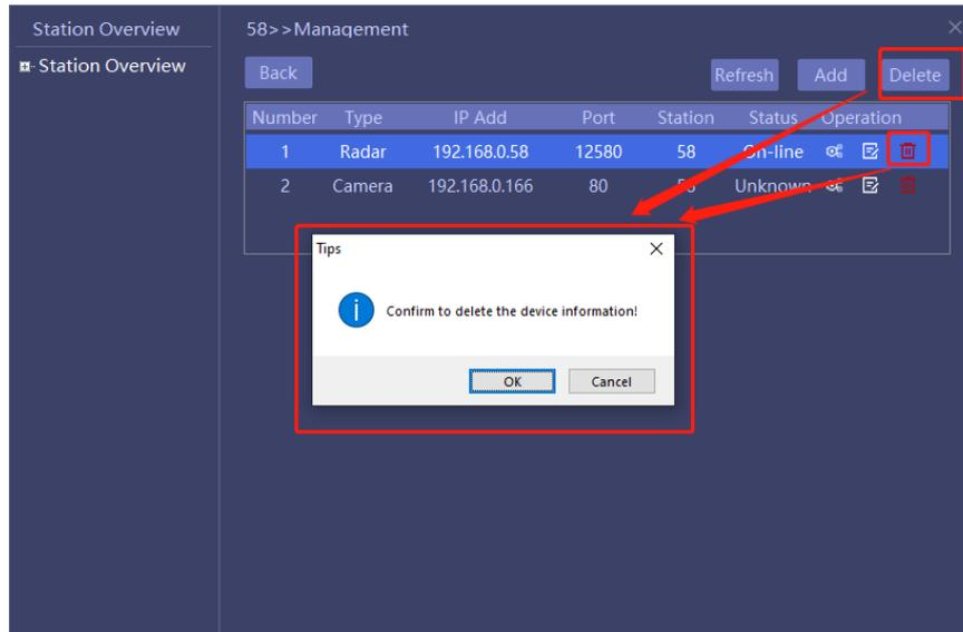
Figure 23Deleting the device
